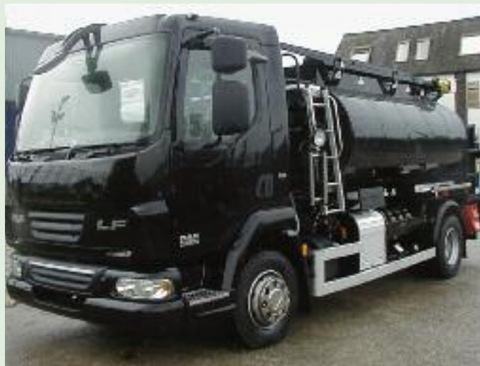
A specialist lube tanker supplied to New Era Oil in Harlow, equipped to carry 5x1000 litres.
