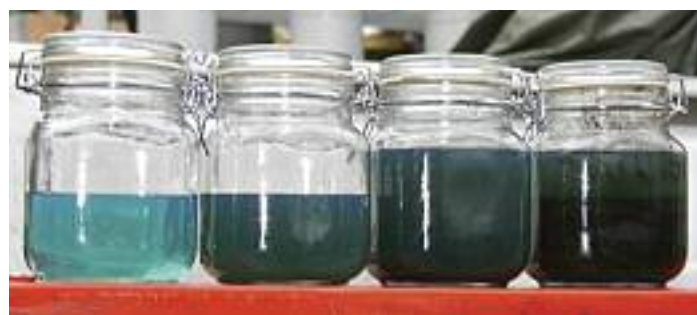
In Thailand, where petrol is dyed blue, the effects of E&S's filtering on product are obvious. The fuel starts off a sludgy black and filtration restores it to its original state.
