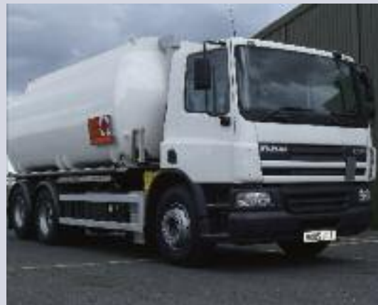
The tank in the photo is a remounted tank from another chassis which was mounted onto the 05 DAF FAN CF75:310 6 x 2 chassis. All the equipment fitted is new.
