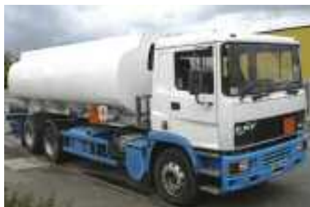
1997 (P) ERF EC12, 34STL 6x2 FUEL TANKER, 20,000 litres aluminium tank, 5 compartments, Alpeco meter, rear lift axle, A/C, tested 26 tons GVW
