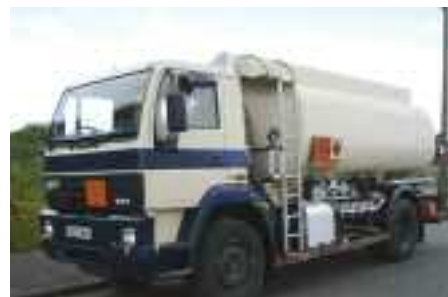
1999 (V) ERF ES6, 22TP2 4x2 FUEL TANKER, 12,400 litres, 4 compartments, Alpeco lectro count meter, tested 18 tons GVW
