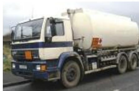
2001 (X) ERF ES8, 30RD3 6x4 FUEL TANKER , 18,500 litres, 5 compartments, Alpeco lectro count meter, top and bottom load, choice 26 tons
