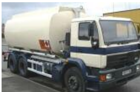
2001 (Y) ERF ES8, 30RD3 6x4 FUEL TANKER , 18,500 litres, 5 compartments, Alpeco lectro count meter, top and bottom load, choice, 26 tons
