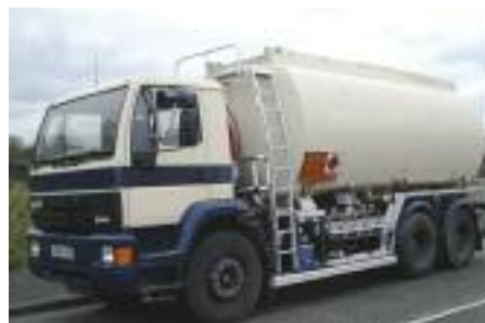
1999/2000 (V) ERF ES8, 30RD3 6x4 FUEL TANKER , 18,500 litres, 5 compartments, Alpeco lectro count meter, top and bottom load choice 26 tons
