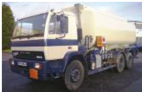
1996 (P) ERF ES8, 28RD3 6x4 FUEL TANKER , 18,500 litres, 4 compartments, top and bottom load, Alpeco meter, tested 26 tons GVW
