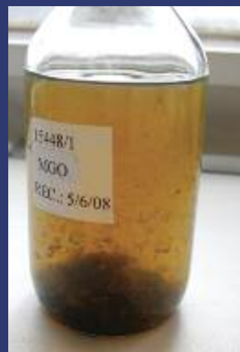
Figure 1. Gas Oil heavily contaminated with microorganisms. Note the turbidity of fuel and soft deposit of microbial growth. When the fuel is disturbed this 'sludge' disperses throughout the fuel.
